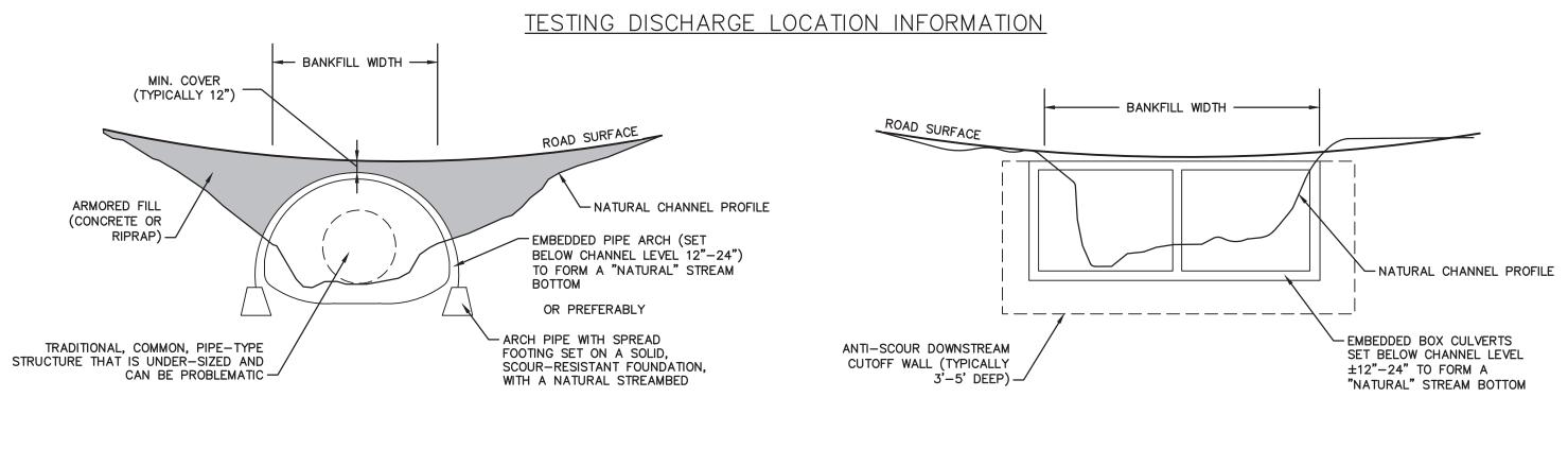
"STREAM SIMULATION" EMBEDDED ARCH OR PIPE-ARCH CULVERTS
