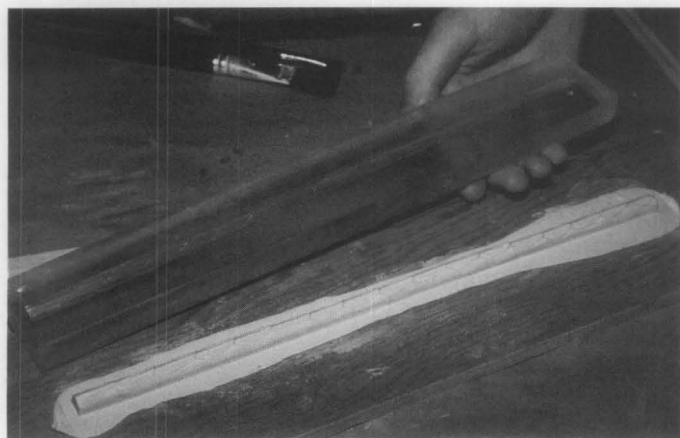
Figure 6. This finished length of compo molding is stuck to its pressing board. The newly made piece will be sliced off the board, then applied. Photo: Jonathan Thornton.
