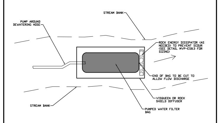
NOTE: THIS DETAIL ONLY APPLIES TO DEWATERING ACTIVITIES AT STREAM CROSSINGS WHERE THE PUMP-AROUND (DAM AND PUMP) METHOD IS SPECIFIED. THIS DETAIL DOES NOT APPLY TO THE HANDLING OF SEDIMENT LADEN WATER.
