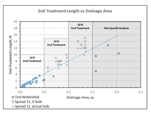
For what is likely to be the most commonly encountered drainage area of less than 0.5 ac (based upon this detailed analysis for Spread 8), the installed end treatment length will be a minimum of 2.5 times longer than necessary.
