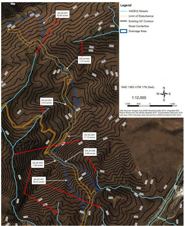
Figure 3. Giles County Drainage Area Delineation Example
